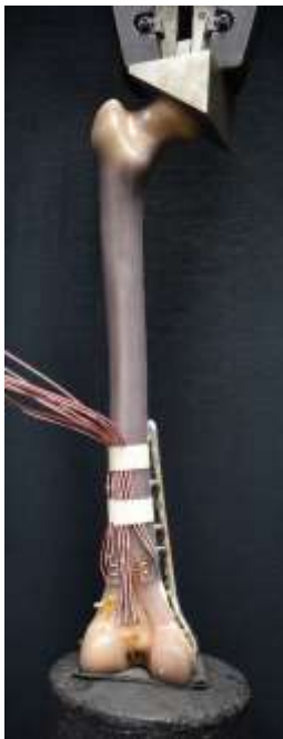
Figure 2. Biomechanical testing setup with strain gauges attached to the posterior distal femur at locations of greatest stress concentration as determined by photostress analysis.
