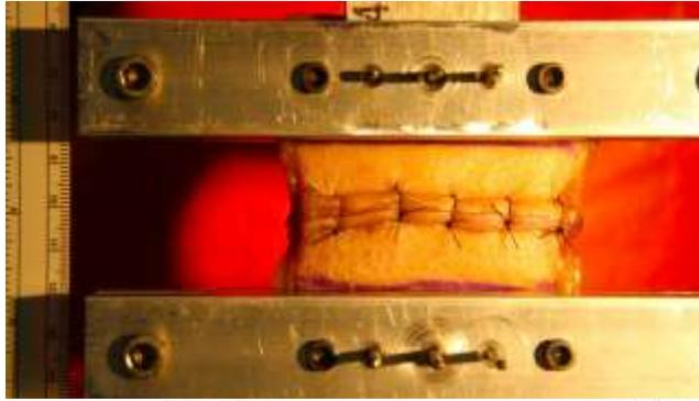
Figure 1. Lindeque locking stitch pattern on cadaveric skin sample being held by serrated grips on the Instron servo-hydraulic system for tensile testing.
