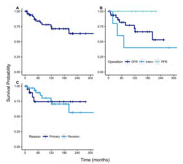
**Figure 1 - Kaplan-Meier survival curves for mechanical failure of endoprosthetic stems with cross pins**. (A) Mechanical failure for all endoprosthesis, (B) by type of reconstruction for three most common operations, (C) by indication, either primary resection or revision.
