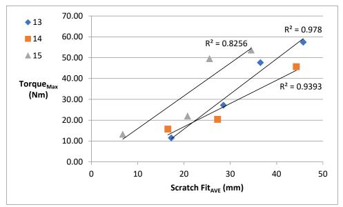
Figure 2. Peak Torque vs. Scratch Fit separated by stem size.
