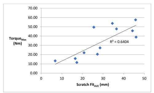
Figure 1. Peak Torque vs. Scratch Fit (all stems).
